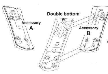
Based on the tilt to be provided, before fastening to the wall, insert **Accessory A** (to provide a tilt of 5° to the left) or
